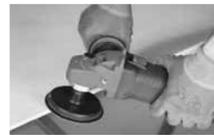
Diamond Blades for simultaneous cutting and grooving
